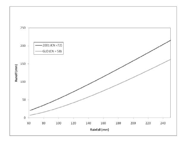
Figure 18. Comparison of rainfall/runoff transformation for the 2001 and GLO land covers using the Curve Number methodology
