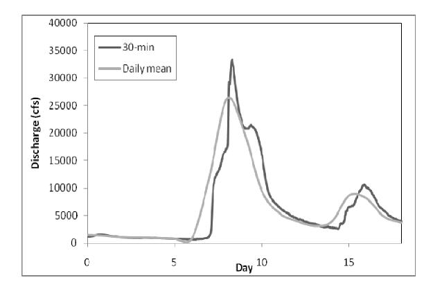
Figure 35. Comparison of hydrographs for the May of 2004 flood event at Elkader using different time steps
